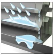
Drains on the front edges of the slats divert water to the sides and out at the bottom of the grille.
